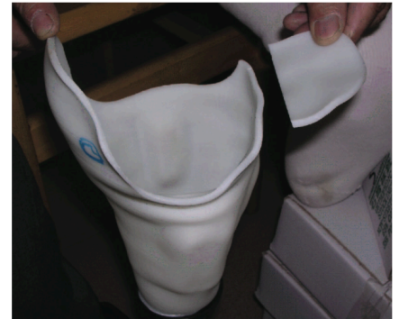
Breakage of socket along forming layer (5)
